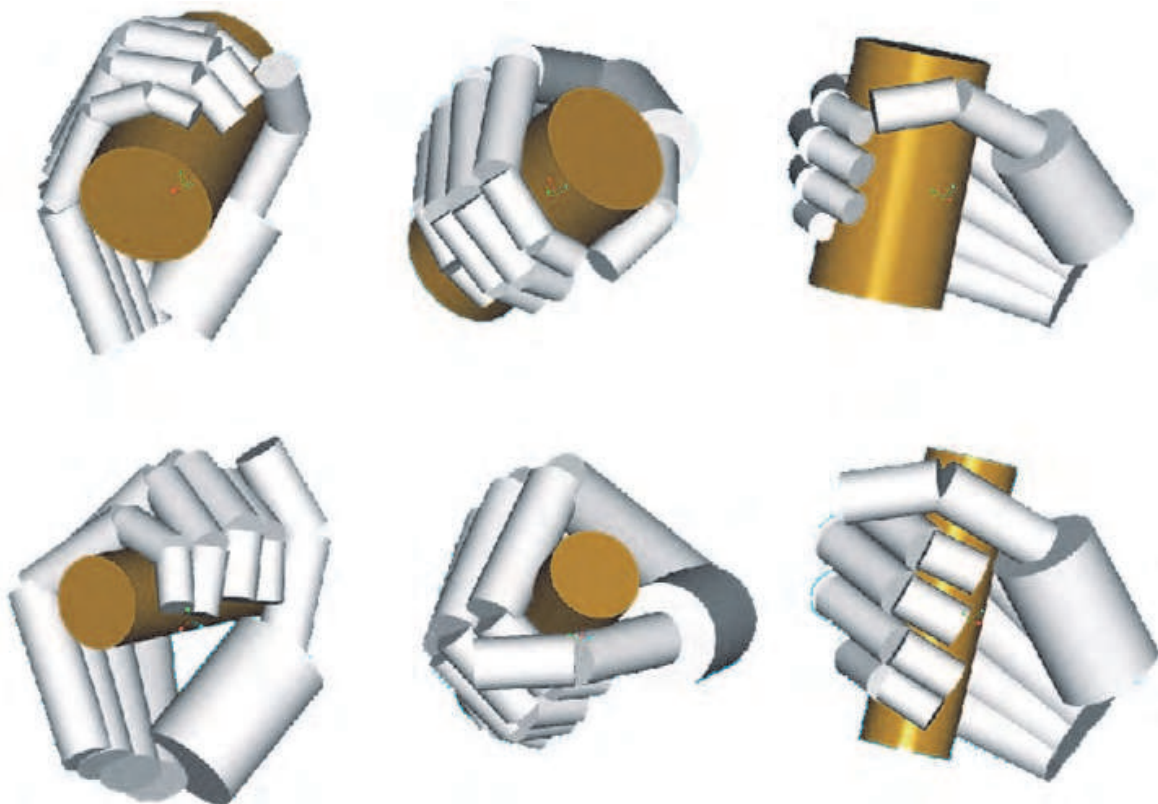
Fig. 1. Different views of the geometric model used in Sancho-Bru et al. (2003a) simulating a hand gripping two cylinders of different diameters.
