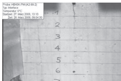
Figure 7. Video image during crack growth.
