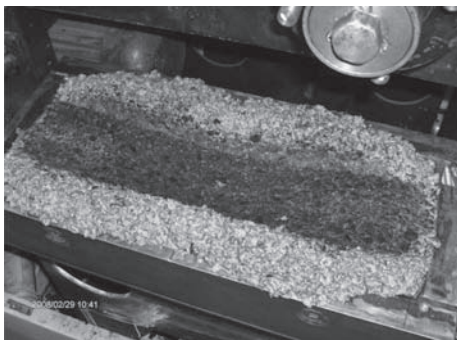
Figure 9. Rutting of the specimen compacted at the “wet side” after a mere 2000 wheel passes (placement void ratio e = 0.18 ).
