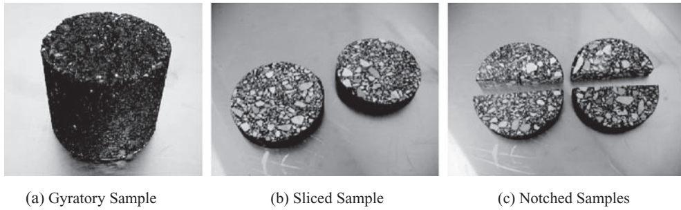
Figure 2. Notched sample preparation steps.
