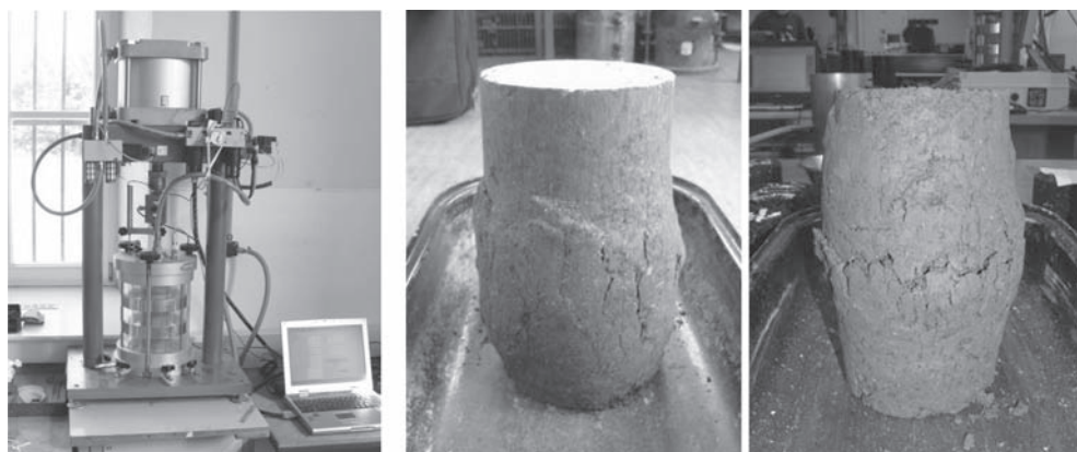
Figure 5. Cyclic triaxial equipment by EN 13286-7 at TU Brno and destroyed testing specimens.
