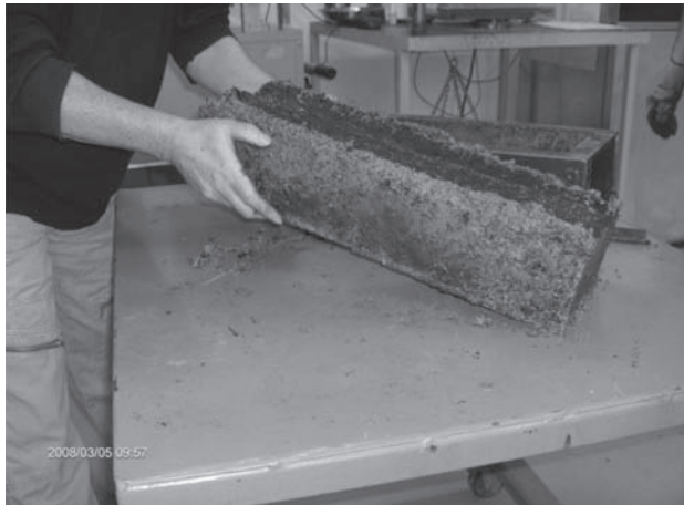
Figure 8. Hard specimen compacted at the “dry side” after rutting test (placement void ratio e = 0.18 ; 60 000 wheel passes).
