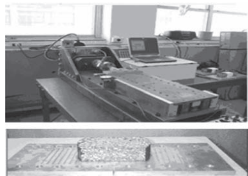
Figure 3. The Overlay Tester (OT) and specimen setup.
