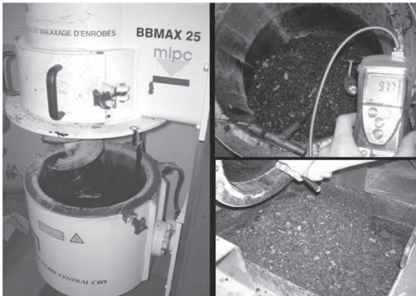
Figure 3. Mixer used for the manufacturing of LEA ® high-modulus mixtures (95°C) and corresponding HMAs (160–180°C) at the EIFFAGE Travaux Publics research centre in Ciry-Salsogne (France).
