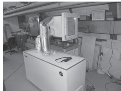
Figure 9. Climate chamber fed from cooling reservoir.
