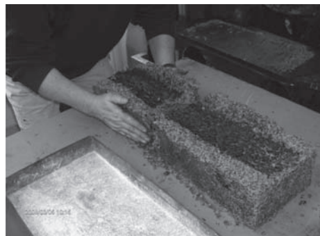
Figure 10. A “soft” consistency of the specimen compacted at the “wet side” after the rutting test (placement void ratio e = 0.18 ).
