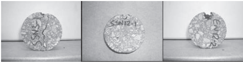
Figure 5. Failure modes for ITFT specimens.
