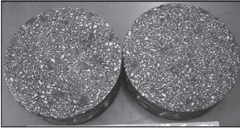
Figure 4. Ottawa sand mix conditioned in NaOH for 7 days at 80°C, showing no gel formation, expansion or cracking.
