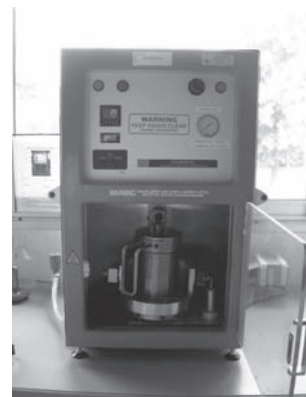
Photo 2. Gyropac press used to make specimens.
