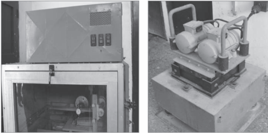
Photograph 5. Wheel tracking machine and vibrate compression unit.
