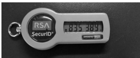
FIGURE 8.9 RSA secure ID token. (Image republished from f-secure.com blog 2011. Used with permission.)
