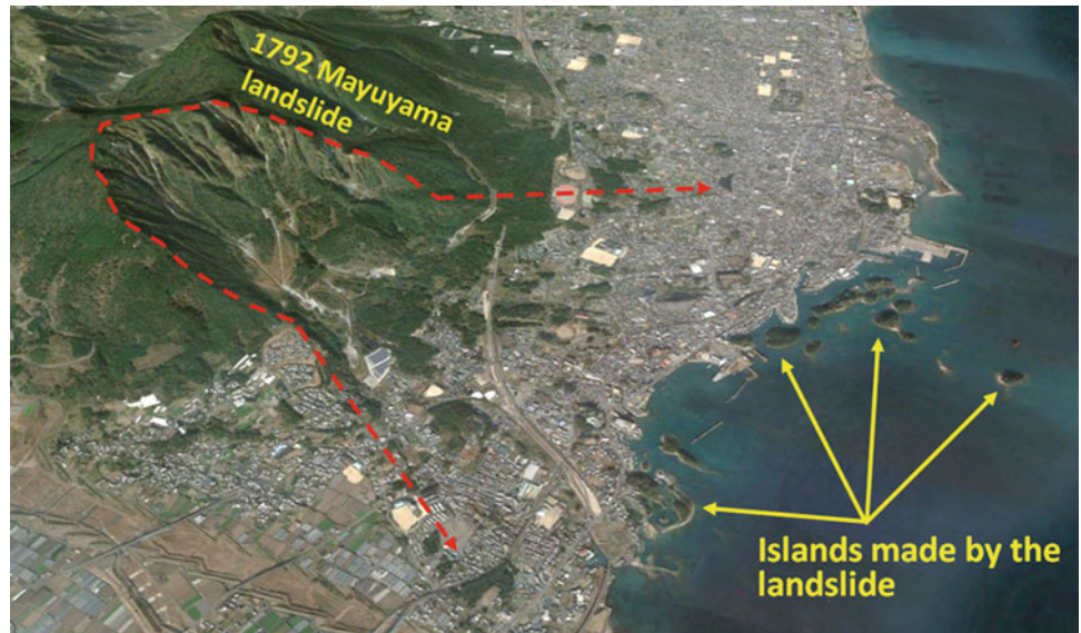
Fig. 28 Google Earth image depicting the Mayuyama landslide and the islands formed as a result of the landslide (modified from Sassa and Dang 2018)
