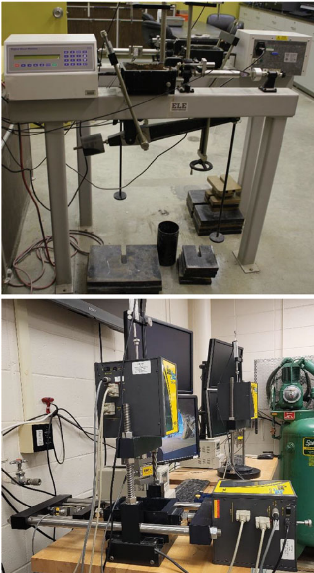
Fig. 8 Pictures of direct shear devices that apply normal stress using (top) weights placed on loading arm and (bottom) pneumatic system
