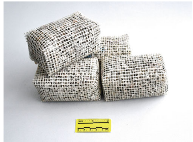
Fig. 6 Photo of gabion model elements
