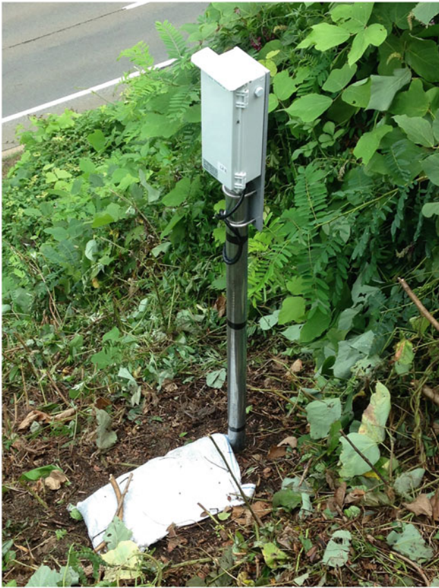
Fig. A.41 Cut slope monitoring Example of sensor installation
