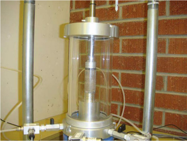
Fig. 13 A triaxial test sample assembly
