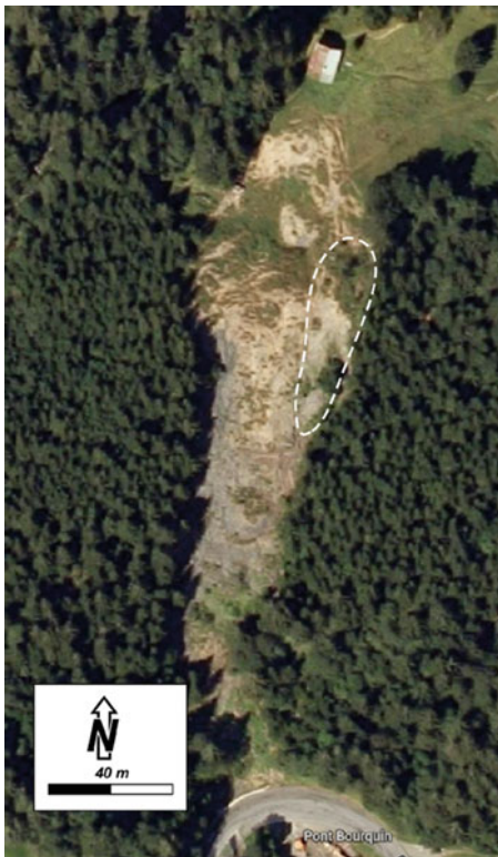
Fig. 14 The location of the unstable zone on the landslide (white dashed line) and the national road that can be affected
