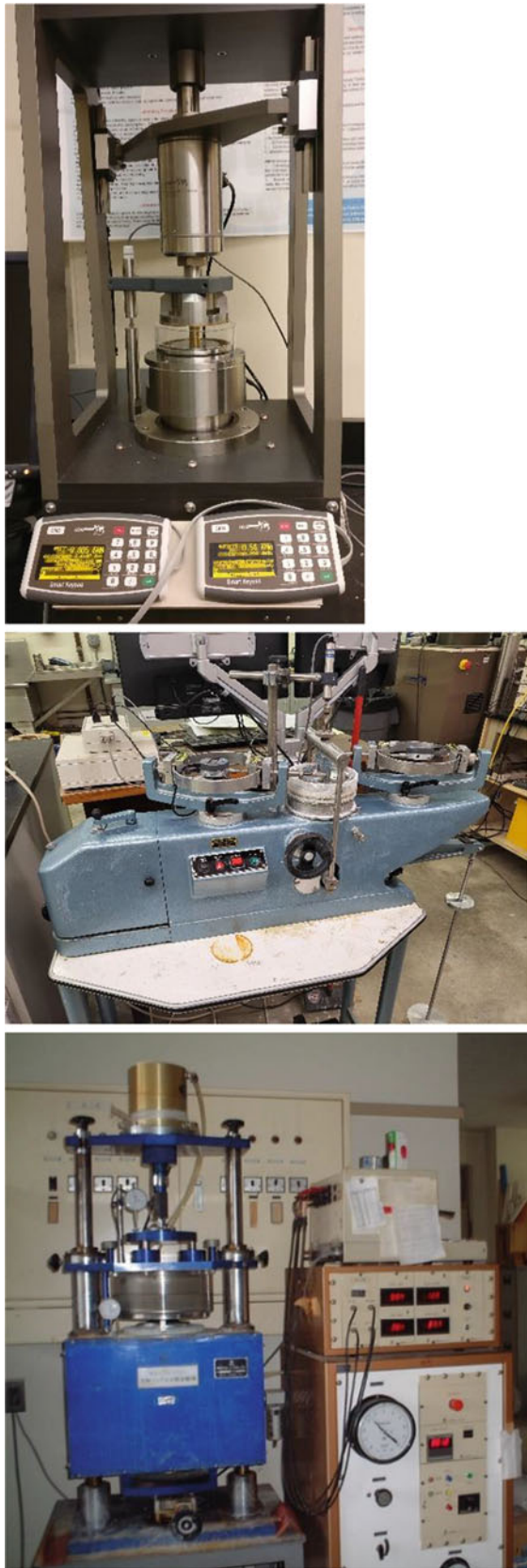
Fig. 28 Different types of ring shear devices available in practice
