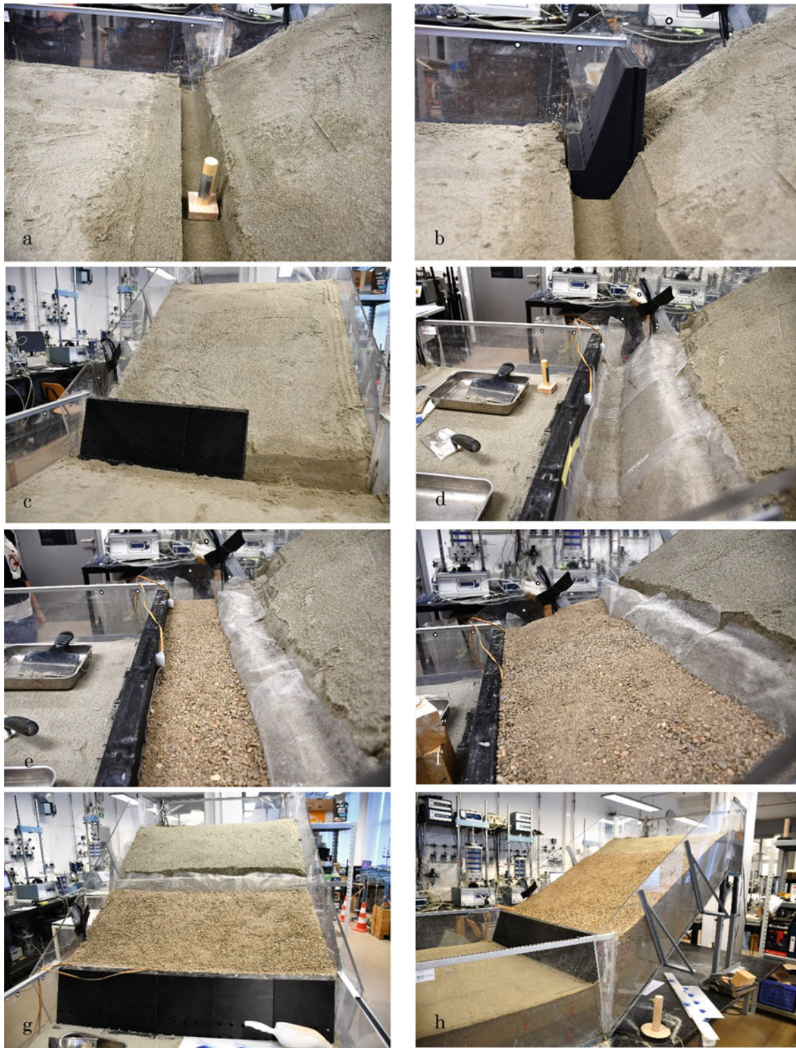
Fig. 8 Installation of the gravity wall and buttressing embankment behind the wall into the prepared sandy slope: (a) excavated foundation pit and installed element of the gravity wall, (b) first wall element installed in the foundation pit, (c) a view at the partially installed wall in the foot of the slope, (d) excavation for backfill behind the wall with
