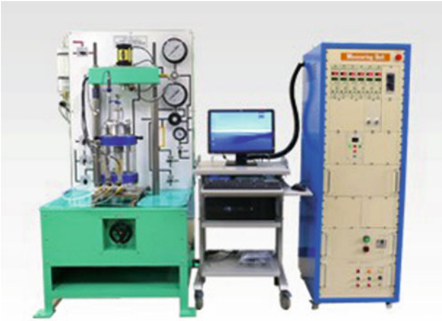
Fig. A.20 Cyclic triaxial testing machine
