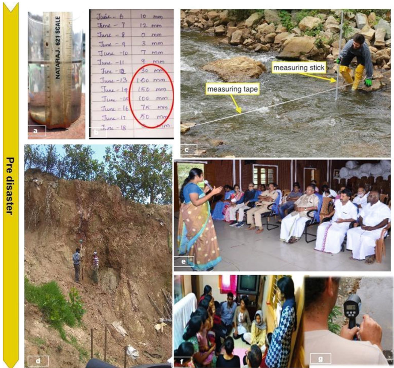
Fig. 4 Implementation of the proposed framework in the pre-disaster period. (a). Measuring rainfall using manual rain gauges by school children. (b). The intensification of rainfall is shown from the data collected by kids in Munnar. (c). Live-in labs students measuring the cross-section of the river in low flow time. This was useful for estimating river discharge (cross-section *height * velocity). (d).
