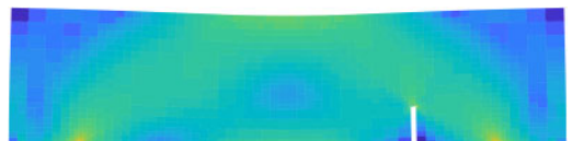
Figure 11. Stress field for the adaptive mesh refinement.
