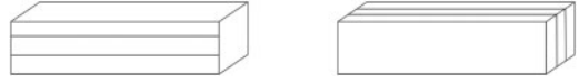
Figure 6. Horizontal and vertical orientation of the 3DPC samples parallel to the layers.
