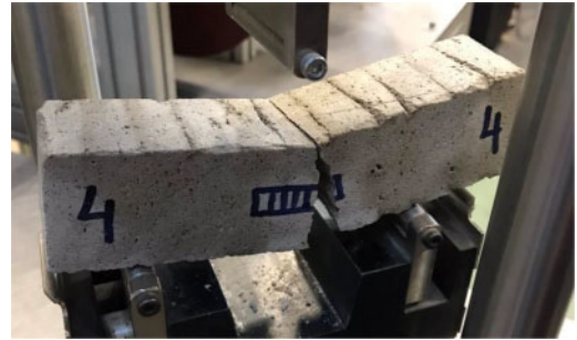
Figure 7. 3-point bending test of the sample with transverse raster orientation (series 1).
