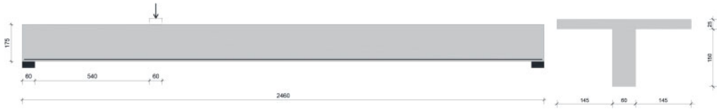
Figure 8. Geometry and loading configuration of set8, dimensions in [cm].
