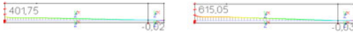
Figure 9. Normal forces into the reinforcement for test G1 (left) and G2 (right), simply supported conditions.
