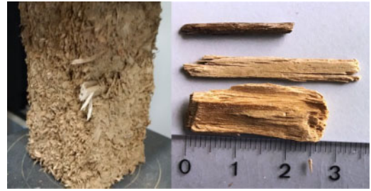
Figure 6. Specimens of adobe with large wood reinforcement visible on the surface (left) and example of fibre geometrical properties revealed in granulometry test (right).
