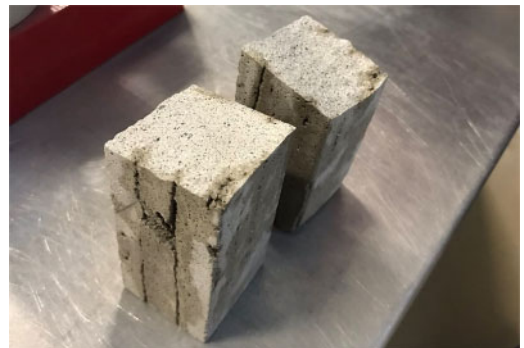
Figure 5. Water penetration in 3D printed concrete sample.
