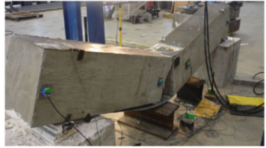
Figure 13. Experimental failure of SP1-2 beam.
