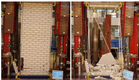
Figure 4. Failure pattern of masonry wall in the TUDCOMP20 experiment before collapse (left) and after collapse (right).
