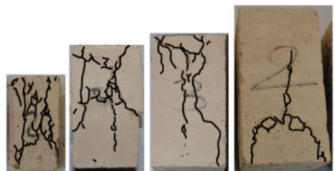
Figure 5. Typical cracking patterns for the different sizes (A-D).
