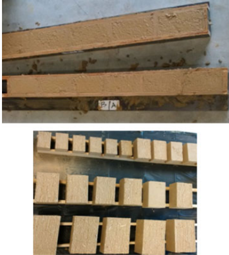
Figure 2. Poured mortar (top) and air drying specimens (bottom).
