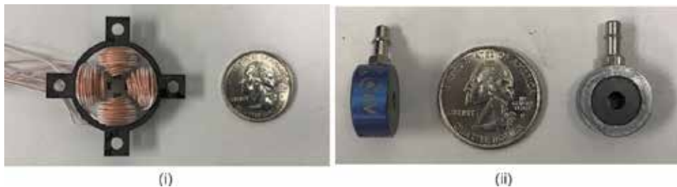
Figure 12. (i) Stator prototype with windings (left). (ii) aerostatic bearings used in the prototype (right).
