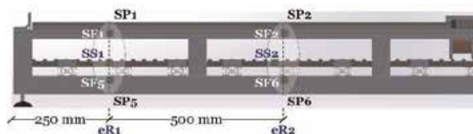
Figure 10. Placement of accelerometers at the left half of the LSRA structure for local response measurements with translator positioned at P2.
