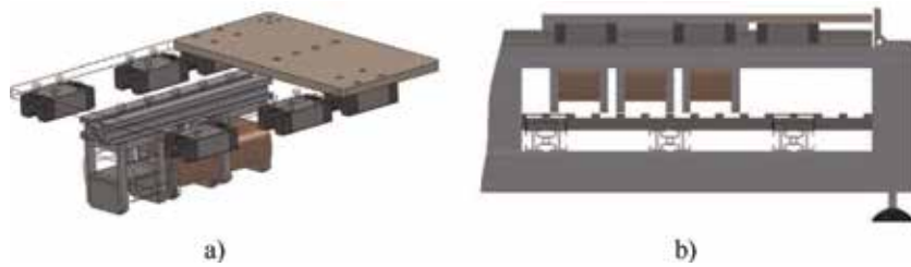
Figure 2. Detailed view of (a) the subassembly of the primary and (b) example of front view position of the translator with full alignment in phase b.
