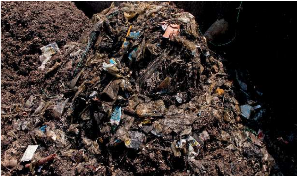
Figure 10.13 Screenings from the Niayes faecal sludge treatment plant in Dakar, Senegal (photo: Linda Strande).
