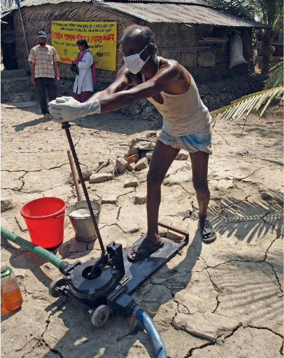
Figure 4.7 Manual diaphragm pump operation in Bangladesh (photo: Georges Mikhael).
