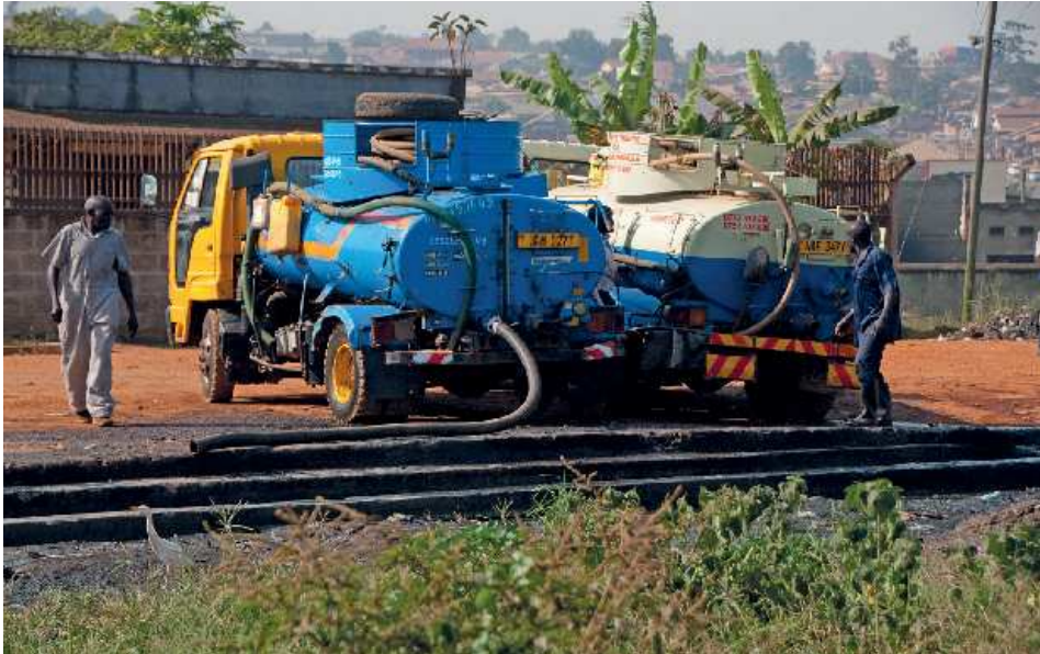
Figure 12.6 Privately owned collection and transport trucks discharging faecal sludge at a receiving facility owned by the municipality, Kampala, Uganda (photo: Linda Strande).
