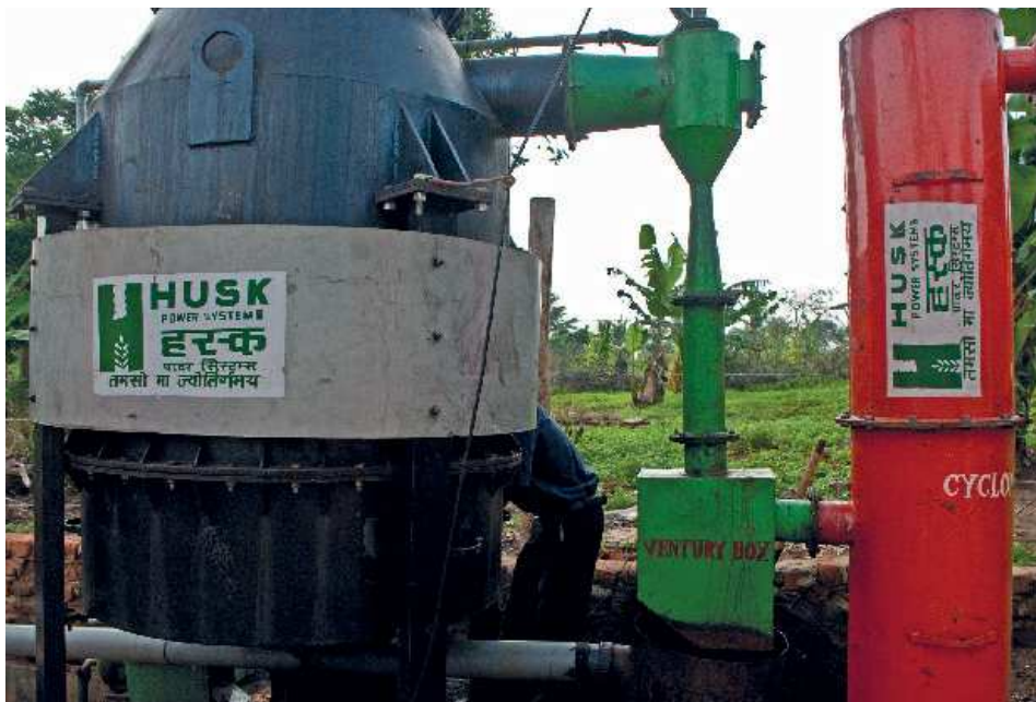
Figure 10.12 Iiribogo gasification project utilising corn husks and sawdust, located in Muduma Sub-county, Mpigi District, Uganda (photo: Linda Strande).
