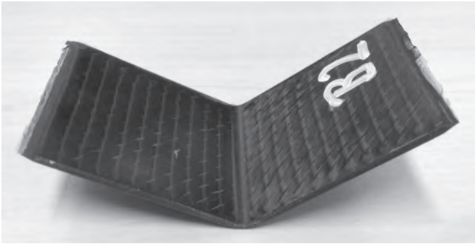
Figure 7.9: L-shaped specimen manufactured using WCM mold and process
