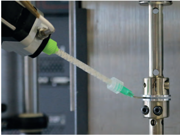
Figure 4.5: Direct injection of the sample into the parallel-plate setup
