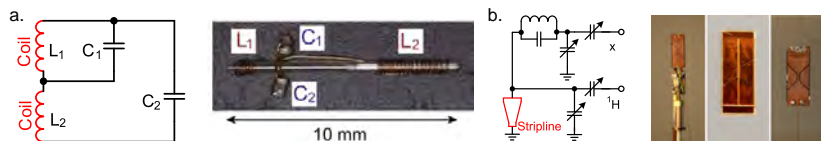
Figure 4.1: a. Inukai [121] suggested a double resonant MACS employing two tank circuits coupled to a MAS coil. b. Oosthoek-de Vries [45] developed trap circuits for a micro-stripline coil. The figure is reproduced from [HD1].
