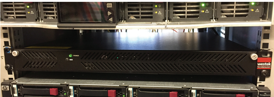
Figure 9.5 IP-based digital exchange for ship-to-shore radio anno 2016.
