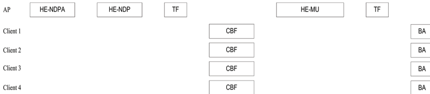
Figure 12.9 Downlink and uplink MU for 11ax.
