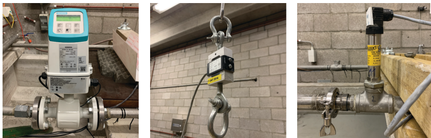
Figure 5.4 Illustration of equipped monitoring devices in the small pumping system (SPS). (Left) Electromagnetic flow meter. (Centre) Load cell from which a container was supported to measure the mass flow rate. (Right) Pressure sensor screwed in a T-connection of the pipeline. Source: originating from [28].
