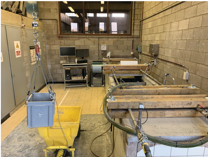
Figure 5.7 Illustration of the SPS used for magneto-rheological pumping experiments. An auger pump is located at the bottom left, above which a container is supported from a load cell to measure the mass flow rate \dot{m} . Source: originating from [6].
