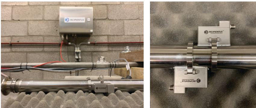
Figure 5.5 Illustration of equipped ultrasonic velocity profiler. (Left) Pipe section on which acoustic transducers are mounted under an inclined angle. (Right) Close-up of acoustic transducers by which ultrasound pulses travel from one sensor to another and back. Source: originating from [6].
