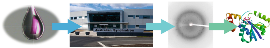
Fig. 1. Structural biology pipeline. Obtaining a crystallised protein is just the beginning. Once a crystal has been grown it is irradiated with X-rays (often at a synchrotron light source). The diffraction images produced at the synchrotron are then used to calculate the atomic structure of the protein.
