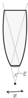
Fig. 1: Illustration of the \gamma -ray microscope based on Heisenberg’s own drawings (Heisenberg 1930). © Provided under the Creative Commons licence by Bryan W. Roberts.
