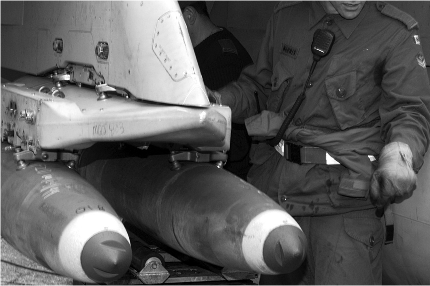
3.4. A Canadian Air Force bomb loader inspects two Mark 82 500-pound General Purpose Bombs, so-called “Dumb Bombs” which are not laser-guided. Photo courtesy of the Department of National Defence.
