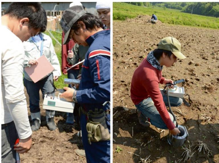
**Fig. 10.6** Measuring ambient radiation doses
