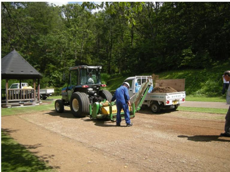
**Fig. 11.1** Practical experiment using a field top maker to decontaminate a park lawn area
