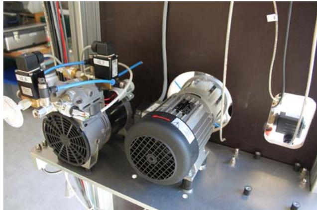
**Figure 4.8** Circulation pump of 1st stage and vacuum pump for draining 1st stage and transferring to 2nd stage.
