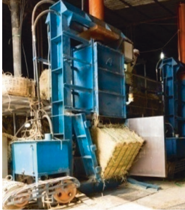
Fig. 2.9 A vertical bale compacting system in operation
