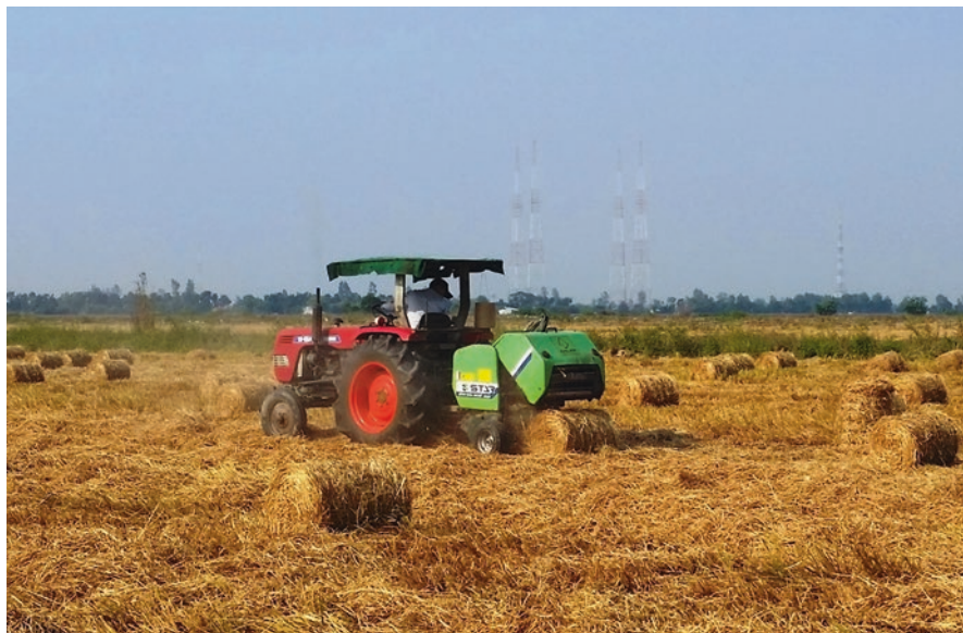
Fig. 2.2 Mechanized straw collection with a small tractor drawn round baler in Vietnam
