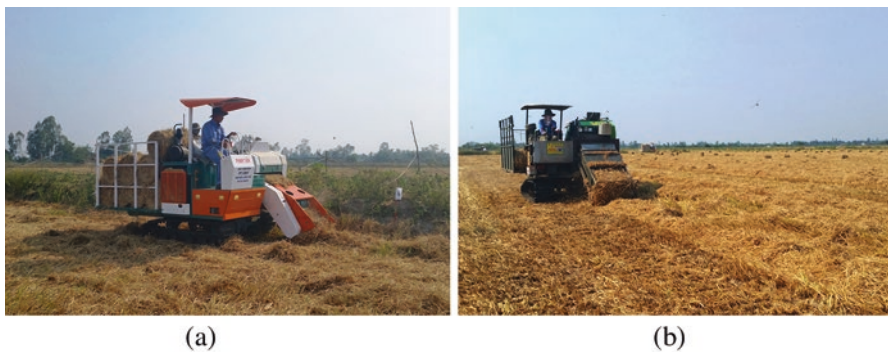
Fig. 2.7 A self-propelled baler (a) and a loose straw collecting machine (b) operating in the field in Vietnam
