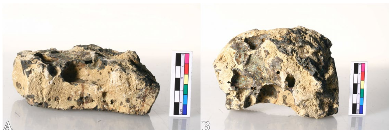
Figure 8. Slag ‘cake’ from the site of Belovode, eastern Serbia, discovered in a context dated to 5200 BC. Compositional analysis revealed lead metal to be the likely product of the smelt (photo CC BY-NC-ND 4.0 M. Radivojević).
