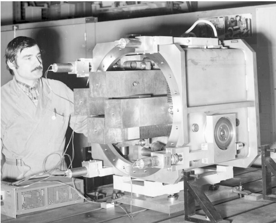
Fig. 2.24 Collimator for extracted beamlines from the SPS at CERN. While not the latest design, this photo shows the metal collimator blocks which, in this model, can be moved to restrict the beam in two directions simultaneously. (Copyright CERN, reused with permission)
