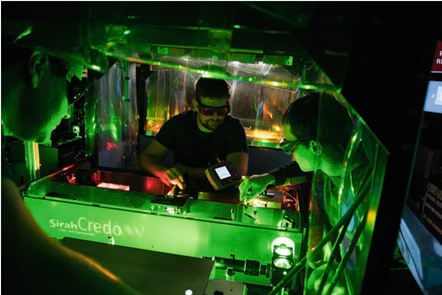
Fig. 2.20 Optical bench in the ISOLDE RILIS laser laboratory. Operators must protect themselves from direct and reflected laser beams with protection glasses. (Copyright CERN, reused with permission)
