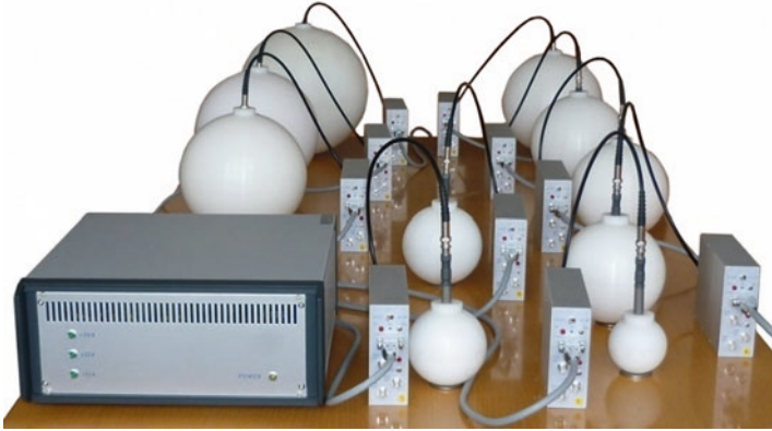
Fig. 3.10 A Bonner-sphere spectrometer consisting of 10 different spheres with amplifiers and data acquisition. [18]
