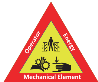
Fig. 4.3 Warning signs against hazards from machines: hand injury, entrapment, crushing, after [1]. (Image source: https://publicdomainvectors.org )
