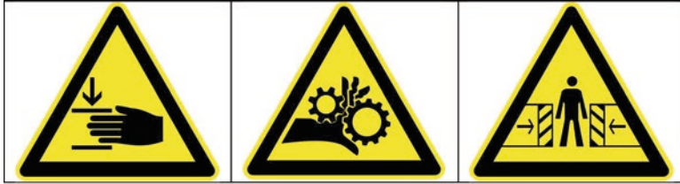
Fig. 4.3 Warning signs against hazards from machines: hand injury, entrapment, crushing, after [1]. (Image source: https://publicdomainvectors.org )
