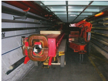
Fig. 2.5 SPS Dipole magnet Left: Cut through the magnet [11]. Right: magnet on a transport carriage. The closed current loops are clearly visible in this perspective. (Copyright CERN, reused with permission)
