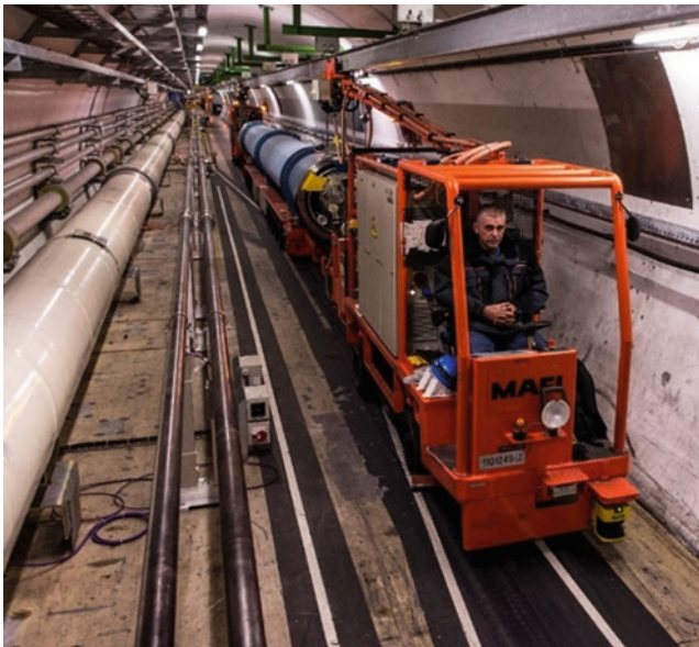
Fig. 4.7 Special vehicle for the transport of superconducting magnets in CERN's LHC tunnel. The vehicle draws electrical energy by the orange catenary from an overhead rail. The vehicle advances by an optical guidance system, following the white line painted on the floor. The white structure to the left is the cryogenic supply line for the superconducting magnets. Copyright CERN, reused with permission
