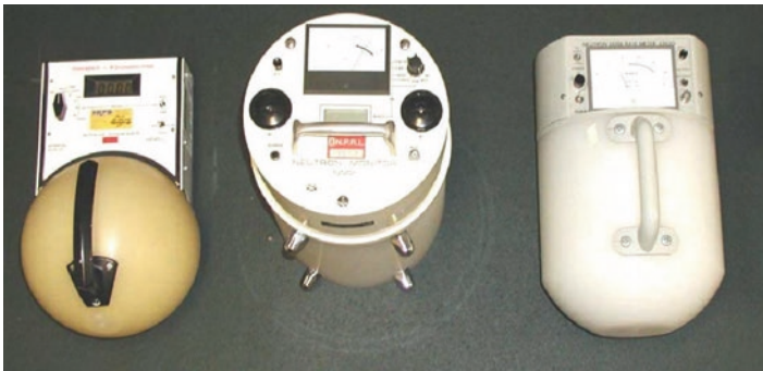
Fig. 3.9 Different commercially available rem-counters. (From [16])
