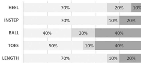
FIGURE 7.46 (a) Rating of nine functional aspects of sports footwear obtained in the benchmarking test with subjects. (b) Fit assessment of the three models by foot zone.
