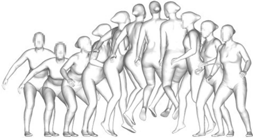
FIGURE 3.44 Sequence of processed body scans during a vertical jump captured with the 4D scanner Move4D.
