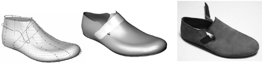
FIGURE 7.38 Shoe prototypes for measuring mechanical properties of the upper material.
