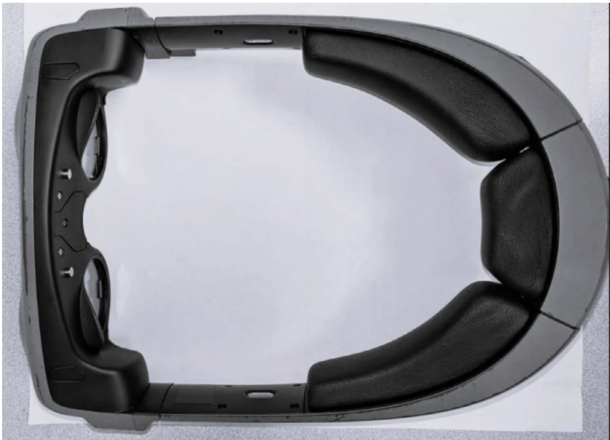
FIGURE 6.31 Headset for which temple arm closing torque was investigated during a trade study.
