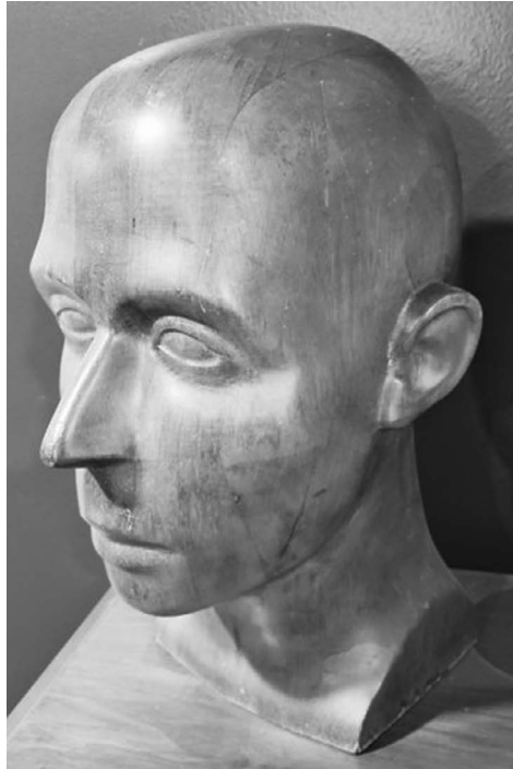
FIGURE 3.35 Size large helmet head form made from wood.
