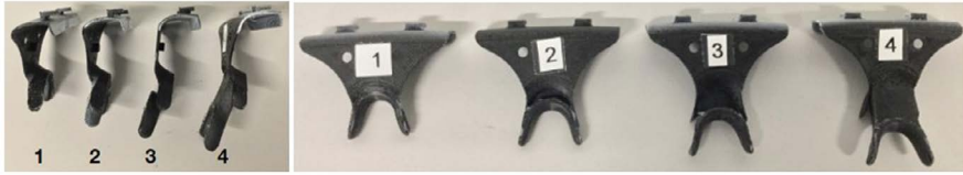
FIGURE 6.12 Early prototype nosepieces used in the design loop fit tests.
