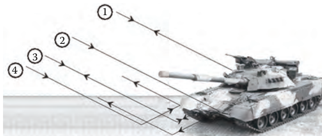
FIGURE 2.48 Basic paths of electromagnetic wave propagation for the case of ground object illumination.
