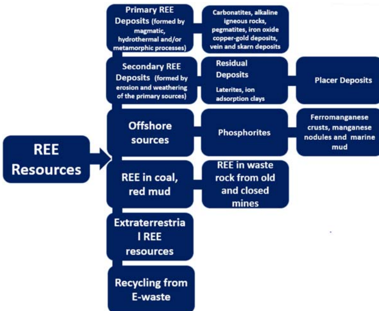
Figure 4.3 Illustrative view of the different types of REE resources (Source: author's design).
