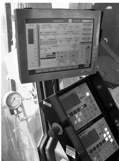
Figure 3.33 Display of multifunctional vibro compaction control panel. (Courtesy of Keller Group plc, London, UK.)
