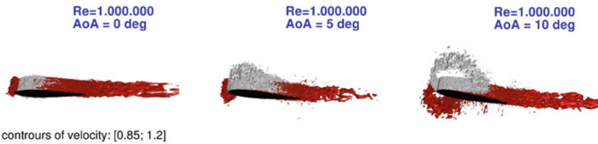
Fig. 2 NACA0012 airfoil at Re = 1 \times 10^6 , from left to right: AoA: 0^\circ , AoA: 5^\circ and AoA: 10^\circ . Simulations are obtained using the incompressible DG solver
