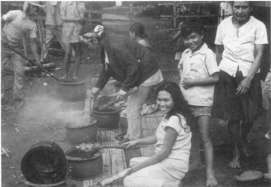
Plate 5. Minahasans of the Lake Tondano region, northern Sulawesi. Pottery still hot from firing is being given a waterproof resin glaze.
