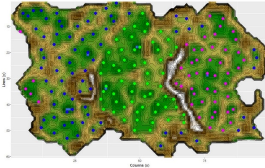
Figure E.20: ESOM projection and U-matrix visualization on Wine data set. The clusters are difficult to separate without the colored labels. Many points are misplaced.
