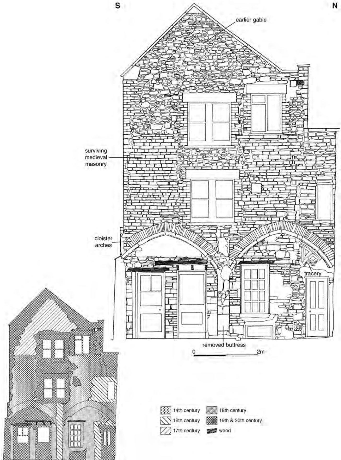
Fig. 13 A survey of the exterior of the rear wall of Church House showing the arches and tracery of the west range of the cloisters (after J. Bryant, 1993)
