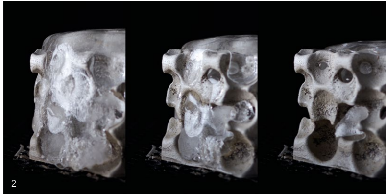
2. Demolding/defrosting of HPFRC hexagon prototype.
