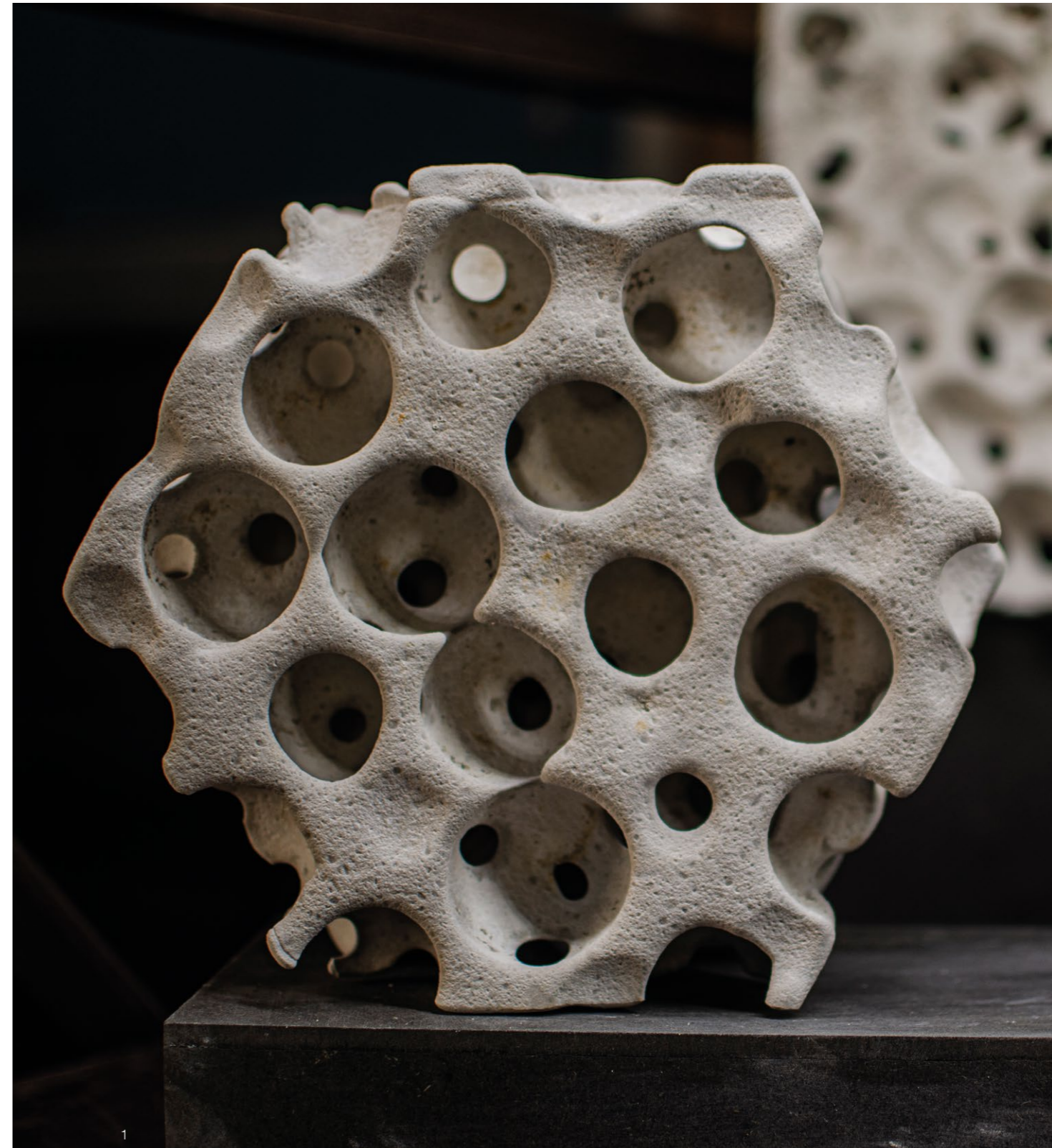
1. A hexagonal prototype of a trabecular HPFRC structure cast using ice aggregate.
