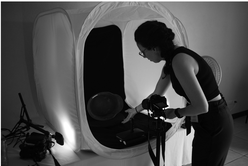
FIGURE 11.7 A demonstration of photogrammetry, used to create 3D models of physical objects in The Enigma of Arrival exhibition.
