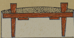
IF THE GROUND WAS MARSHY, WOODEN PILES WOULD BE SUNK AND A TIMBER FRAME WORK USED AS A FOUNDATION
