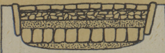
3. LAYERS OF SAND (SOMETIMES CHALK), LARGE STONES FIXED WITH CEMENT AND COMPRESSED GRAVEL. SAND, EARTH & BRICK MIXED TOGETHER. FINAL SURFACE OF STONES OR PEBBLES WELL RAMMED DOWN.
