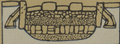
TOWN ROADS HAD STEPPING STONES, AND SOMETIMES CULVERTS WHICH LED OFF WATER TO DRAINS.
