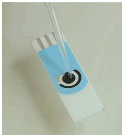
Fig. 8. Screen printed electrode used for biomediator immobilization.
