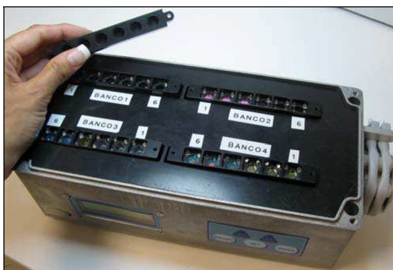
Fig. 7. Biosensing platform set-up consisting of 24 cells able to host an array of several biomediators.
