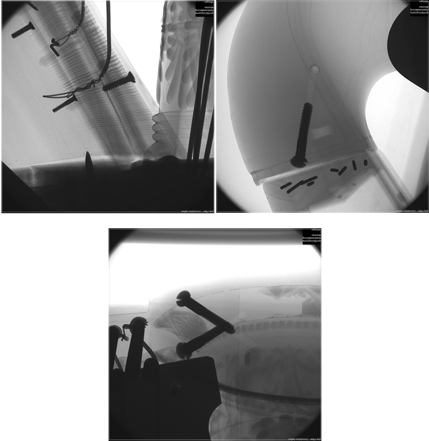
Figure 8. Screws of various sizes on the soundboard, shoulder and capital of Erard N° 2631, housed at the Deutsches Museum, Munich (Inv. No. 16147), revealed during its examination with radiography.
