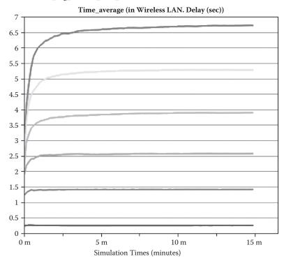
FIGURE 10.8 (SEE COLOR INSERT.) Effect of increasing wireless stations on packet delay of an 802.11g infrastructure network.
