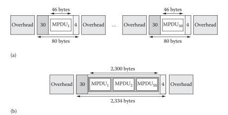
FIGURE 9.4 Protocol overheads for the transmission of short IP datagrams of 46 bytes in length for (a) 802.11b DCF and (b) BUMA $_{nonopt}$ .
