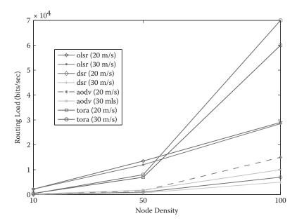
FIGURE 11.41 Routing load versus node density (20 and 30 m/s).
