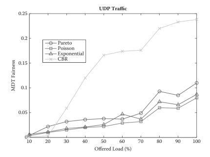
FIGURE 13.7 MDT fairness versus traffic load for UDP (N = 10 stations; packet length: 1,500 bytes; propagation model: shadowing with  $\sigma$  = 7 dB).
