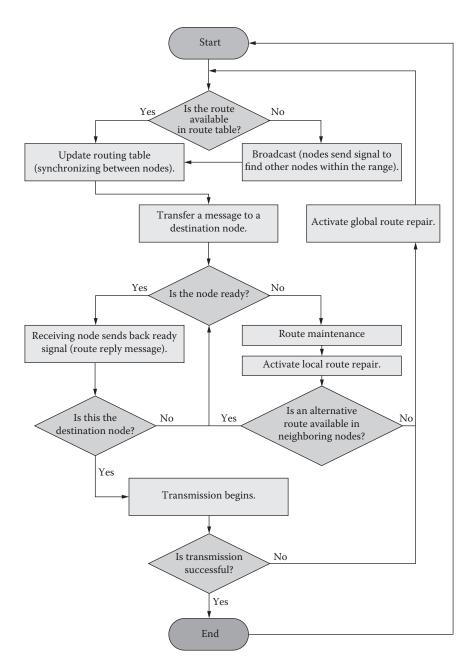
FIGURE 5.5 AODV routing algorithm.
