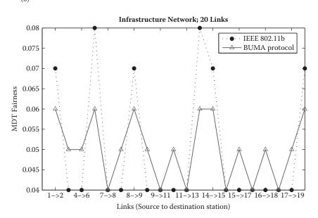
FIGURE 9.12 MDT fairness versus active links of BUMA and 802.11b DCF: (a) ad hoc network and (b) infrastructure network.
