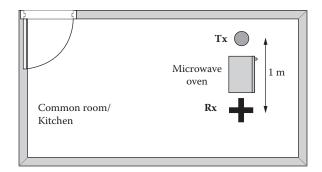
FIGURE 7.19 Effect of microwave oven test (first floor of Environment A). Positions of transmitting and receiving antennas are indicated by ● and +, respectively.
