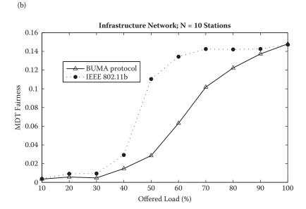
FIGURE 9.13 The effect of offered load on MDT fairness of BUMA and 802.11b DCF: (a) ad hoc network and (b) infrastructure network.
