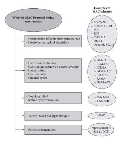
Mechanisms used in the design of representative wireless MAC FIGURE 4.1 protocols.
