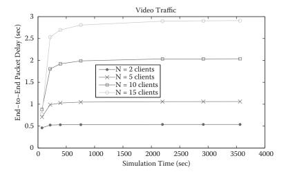
FIGURE 14.10 Effect of increasing the number of wireless video clients on end-to-end packet delay.
