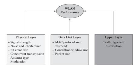
FIGURE 2.3 WLAN performance-limiting factors.
