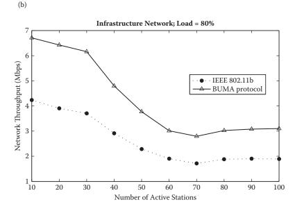
FIGURE 9.9 The effect of the number of active stations on network throughput of BUMA and 802.11b DCF: (a) ad hoc network and (b) infrastructure network.
