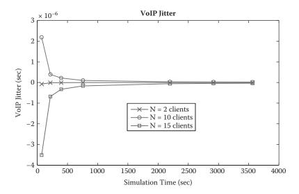
FIGURE 14.7 Effect of increasing the number of VoIP wireless clients on jitter.
