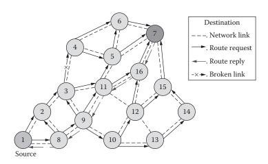
FIGURE 5.4 (SEE COLOR INSERT.) AODV routing mechanism.
