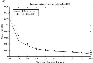
FIGURE 9.14 The effect of the number of active stations on MDT fairness of BUMA and 802.11b DCF: (a) ad hoc network and (b) infrastructure network.
