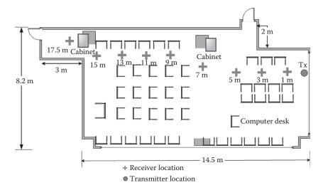
FIGURE 7.20 Floor plan of Environment B indicating the measurement locations for scenario 1 (802.11b ad hoc network).
