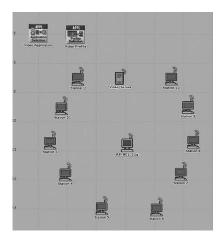
FIGURE 14.5 OPNET representation of an 802.11g infrastructure network with a wireless video server, 1 AP, and 15 clients.
