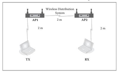
FIGURE 10.4 WDS with AP mode configuration.
