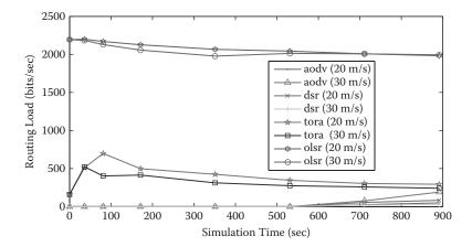
FIGURE 11.16 Routing load versus simulation time (N = 10, NS = 20 and 30 m/s, PL = 1,000 bytes).
