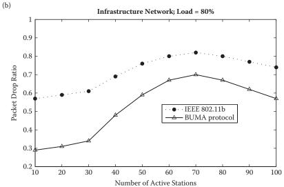
FIGURE 9.15 The effect of the number of active stations on the packet drop ratio of BUMA and 802.11b DCF: (a) ad hoc network and (b) infrastructure network.
