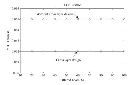
FIGURE D.7 MDT fairness with and without CLD for TCP traffic.
