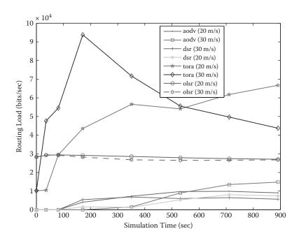
FIGURE 11.24 Routing load versus simulation time (N = 100, NS = 20 and 30 m/s, PL = 1,000 bytes).
