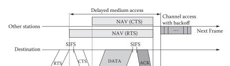
FIGURE 2.8 DCF RTS-CTS method (four-way handshaking). (From J. F. Kurose and K. W. Ross, *Computer Networking: A Top-Down Approach*, 4th ed., New York: Addison Wesley, 2008.)
