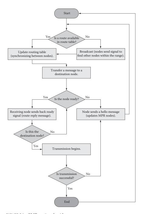
FIGURE 5.1 OLSR routing algorithm.
