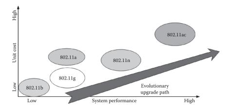
FIGURE 15.1 An evolutionary path of various 802.11 WLANs.
