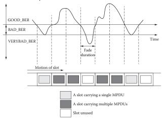
FIGURE 12.9 Illustrating the basic operation of the CLD algorithms.
