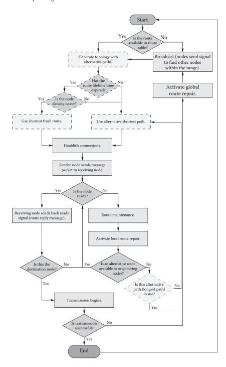
FIGURE 5.8 Proposed P-AODV algorithm.
