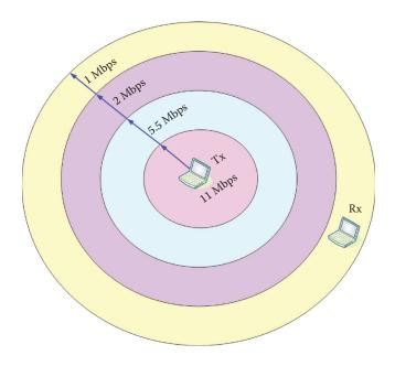
FIGURE 2.4 Data rate and coverage area in 802.11b.
