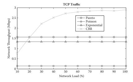
FIGURE 13.2 Mean throughput versus traffic load for TCP traffic (N = 10 stations; packet length: 1,500 bytes; propagation model: shadowing with  $\sigma = 7$  dB).
