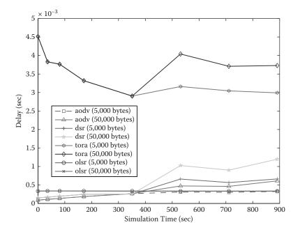
FIGURE 11.34 Packet delay versus simulation time (N = 50, NS = 30 m/s, PL = 1005,000 and 50,000 bytes).
