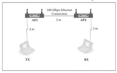
FIGURE 10.5 AP mode with Ethernet connection.
