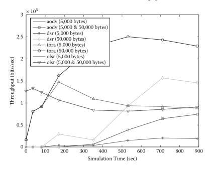
FIGURE 11.35 Average throughput versus simulation time (N = 100, NS = 30 m/s,  $PL = 5{,}000$  and 50,000 bytes).
