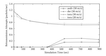
FIGURE 11.21 Retransmission versus simulation time (N = 50, NS = 20 and 30 m/s, PL = 1,000 bytes).
