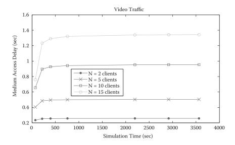
FIGURE 14.11 Effect of increasing the number of wireless video clients on channel access delay.
