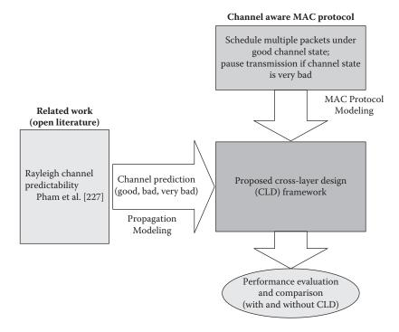
FIGURE 6.1 Developing the proposed CLD framework for WLANs.
