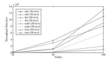
FIGURE 11.40 Throughput versus node density (20 and 30 m/s).
