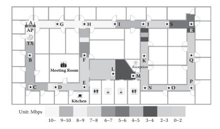
FIGURE 15.2 Layout of floor 1 of the Duthie Whyte (WY) building and measurement locations. Measurement results in a throughput map.
