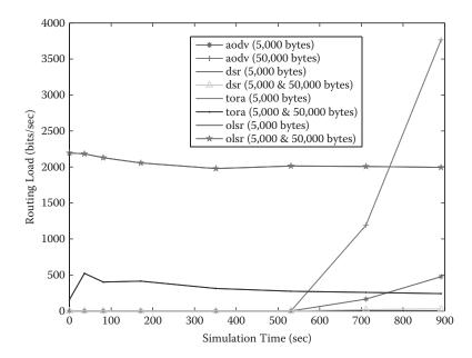
FIGURE 11.28 Routing load versus simulation time (N = 10, NS = 30 m/s, PL = 5,000 and 50,000 bytes).
