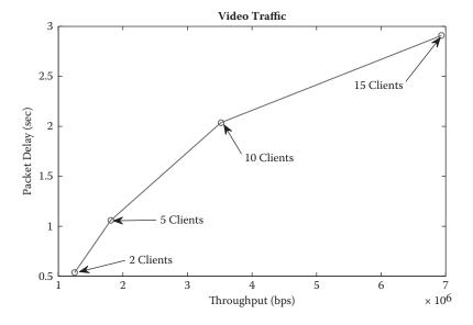
Mean packet delay versus throughput characteristics of video traffic.
