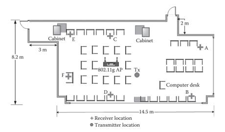
FIGURE 7.21 Floor plan of Environment B indicating the measurement locations for scenario 2 (802.11g infrastructure network).
