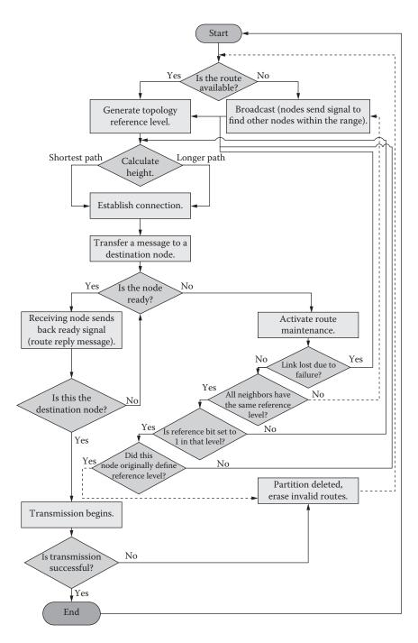
FIGURE 5.7 TORA routing algorithm.
