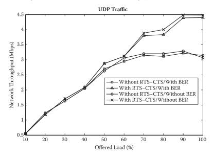
FIGURE 12.2 Network throughput versus load for UDP traffic.
