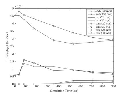
FIGURE 11.19 Throughput versus simulation time (N = 50, NS = 20 and 30 m/s, PL = 1,000 bytes).
