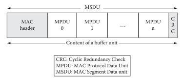
FIGURE 9.2 Frame structure of the BUMA protocol.
