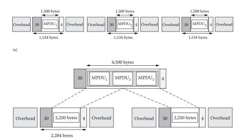
FIGURE 9.5 Protocol overheads for the transmission of large IP datagrams of 1,500 bytes in length for (a) 802.11b DCF and (b)  $BUMA_{opt}$ .
