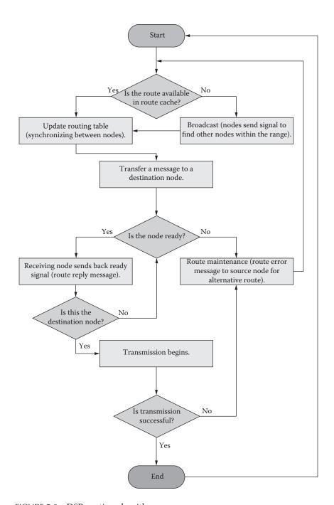
FIGURE 5.3 DSR routing algorithm.
