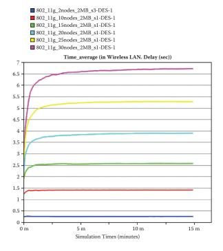
FIGURE 10.8 Effect of increasing wireless stations on packet delay of an 802.11g infrastructure network.
