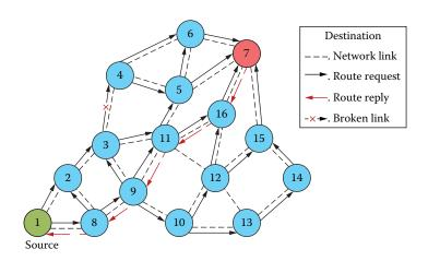
FIGURE 5.4 AODV routing mechanism.
