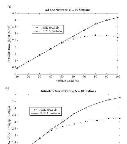
FIGURE 9.8 The effect of offered load on throughput of BUMA and 802.11b DCF: (a) ad hoc network and (b) infrastructure network.
