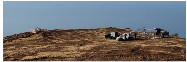
Fig. 9 The collocation of a GNSS CORS and a corner reflector (descending mode) in the ALEV site
