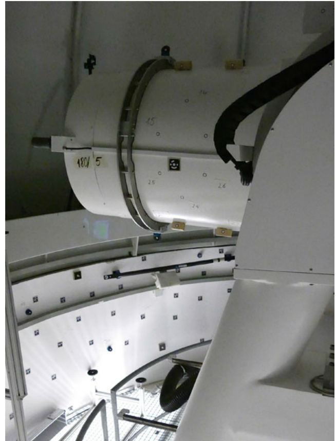
Fig. 3 Prepared telescope and photogrammetric reference frame with scale bar at the dome wall
