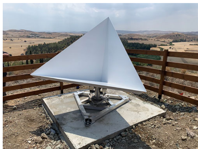
Fig. 7 The triangular trihedral Corner Reflector (CR) type deployed at the CyCLOPS permanent sites
