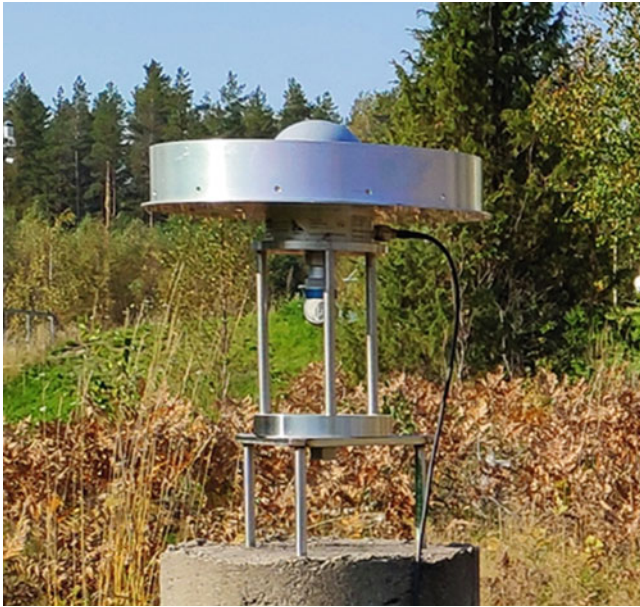
Fig. 6 The seamless adapter for GNSS antenna and prisms at a pillar point
