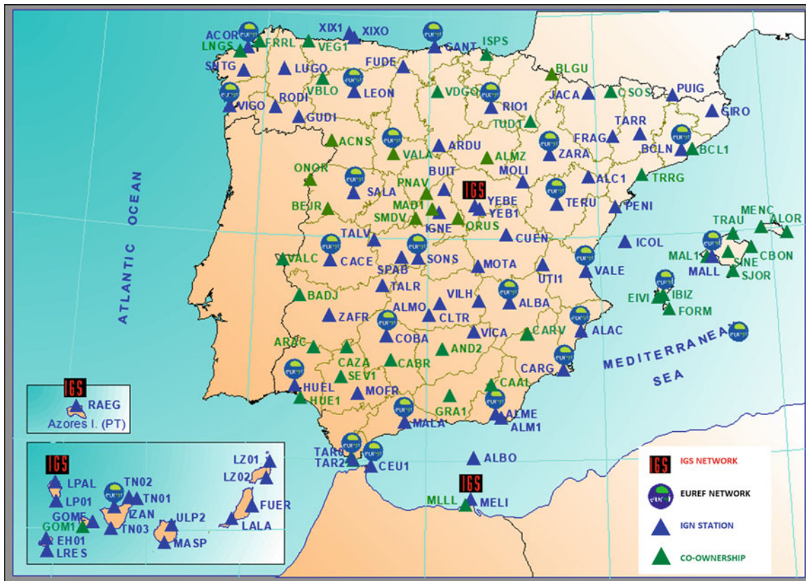
Fig. 2 Spanish National GNSS Permanent Network (ERGNSS). Blue triangles are IGN stations; Green triangles are stations in a joint-ownership
