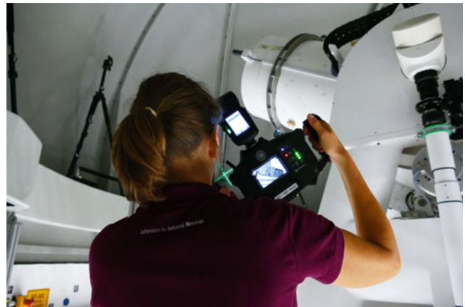
Fig. 2 Close range photogrammetry for SLR reference point determination
