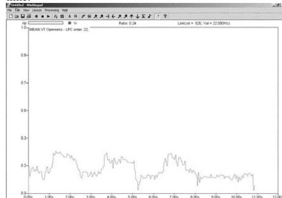
Figure 5: Example display of mean vocal tract area against time for /a:/ sung alternating between a non-projected (lower values) and a projected style (higher values).
