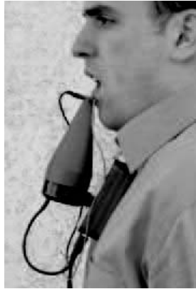
Figure 5: Prototype of the impedance measurement set-up
