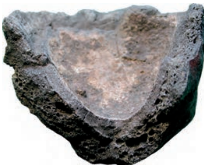
Plate 16. Crucible showing outer coating 2021.
