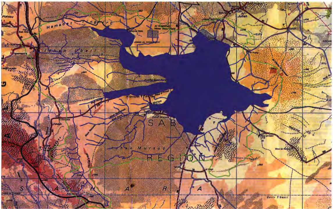
Fig. 2.16. Fazzān palaeolake estimated from Differential GPS heights of known shorelines and GTOPO30 digital elevation model. See text for discussion.
