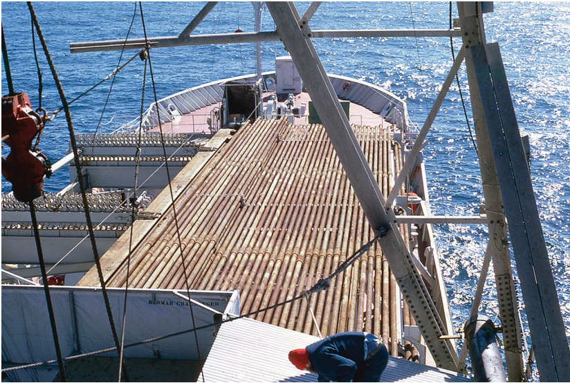
Figure 1.4. Pipe rack on the foredeck of the Glomar Challenger .
