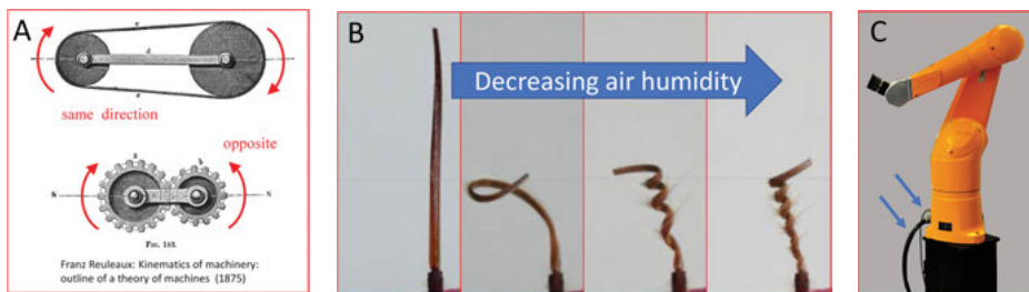
Fig. 6: Degrees of freedom and energy supply in mechanical systems. (A) The right wheel in the system governed by a belt or a gear has no degree of freedom. It has to turn either in the same direction or in the opposite direction to the left wheel. The energy for the movement is transferred directly from the movement of the left wheel. Adapted from: [Reuleaux 1876, p. 262, figs. 182, 183]. (B) The various states of the Erodium awn depend on its water content, which in turn depends on air humidity. © Rivka Elbaum (Hebrew University of Jerusalem) and Peter Fratzl (MPI-CI). As with any material property, the geometric appearance (output) is a direct function of air humidity (input). Hence, the geometric state is completely predictable from the input, in the same way as the rotation direction of the right wheel in (A) is completely predicted by the movement of the left wheel. The corresponding material property has been programmed by the plant during the growth of the awn by a complex arrangement of cellulose fibrils [Abraham et al. 2020]. The energy for the shape change is directly taken from the environment (via water absorption or evaporation). (C) In contrast to (A) and (B), the robotic arm in (C) has several degrees of freedom materialized by its articulations (the photo was edited by Peter Fratzl). The control is delegated to an outside processor and the information needs to be imported through a cable (blue arrow), as does the energy for the movement (second blue arrow).
