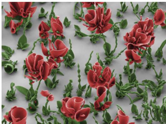
Fig. 4: Gardens of microflowers, complete with leaves, blossoms, and even a few snails, can be sculpted simply by combining two competing chemical precipitation reactions in a beaker and taking advantage of unique reaction-diffusion pathways that result. The size of each microstructure is ~ 100 times smaller than the width of a human hair. © The Aizenberg lab's.
