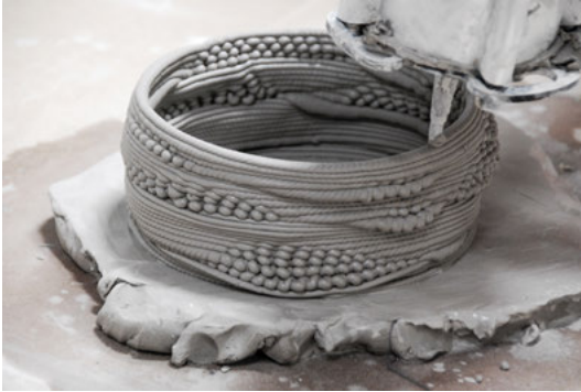
Fig. 1: A clay vessel robotically printed by Co-de-iT as part of the inFORMed matter research project. © Bruno Demasi (reproduced with authorization).
