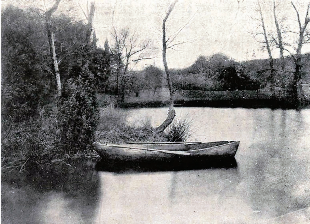
Figure 1.5.1 “Un bateau en ciment armé âgé de 54 ans. Vue du lac de Miraval (A boat in reinforced cement 54 years old. View taken from Miraval Lake)”.
