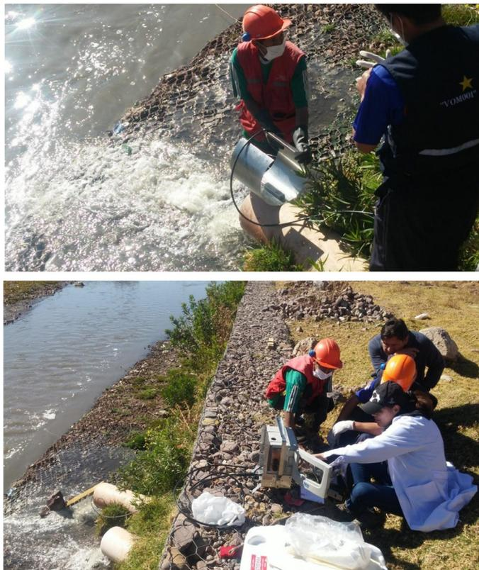
**Figure 3.12** Measuring flowrate with an area velocity digital flow meter, which has ring inserts for different diameter sewers, for the design of a wastewater treatment plant for a small city, Saylla, Peru. Note the second discharge pipe that was not part of the original sewer design and was clandestinely added more recently as a result of rapid population growth. Photos courtesy of CONASIN SRL, Cusco, Peru.
