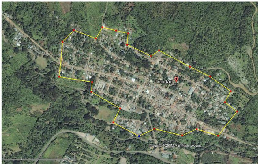
**Figure 3.10** The service area for Trinidad is estimated to be 53.3 ha using Google Earth. In practice, the municipal plans of the city should be used to calculate service areas and lengths of sewer pipes for use in Equations (3.1) or (3.2).
