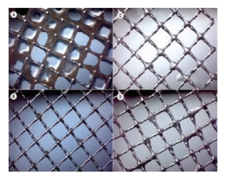
**Figure 11.8** Effect of flushing (at  $0.42 \text{ ms}^{-1}$ ) on biofouling developed at low and high linear flow velocity (0.06 and  $0.31 \text{ ms}^{-1}$ ). Biofilm developed at low linear flow velocity ( $0.06 \text{ ms}^{-1}$ ) before (**A**) and after flush (**B**), and developed at high linear flow velocity ( $0.31 \text{ ms}^{-1}$ ) before (**C**) and after flush (**D**)
