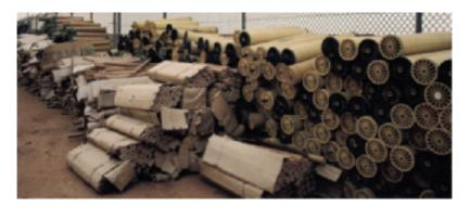
Figure 1.11 Spiral wound reverse osmosis elements and cartridge filters used for polishing RO feed water
