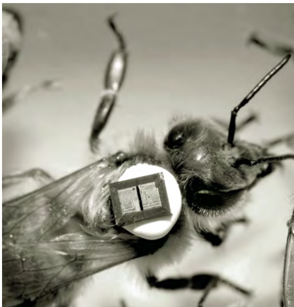
FIGURE 1.6 (See color insert.) Bee with an RFID tag glued to the back side of her thorax. (Reproduced with kind permission of Axel Decourtye, ACTA.)
