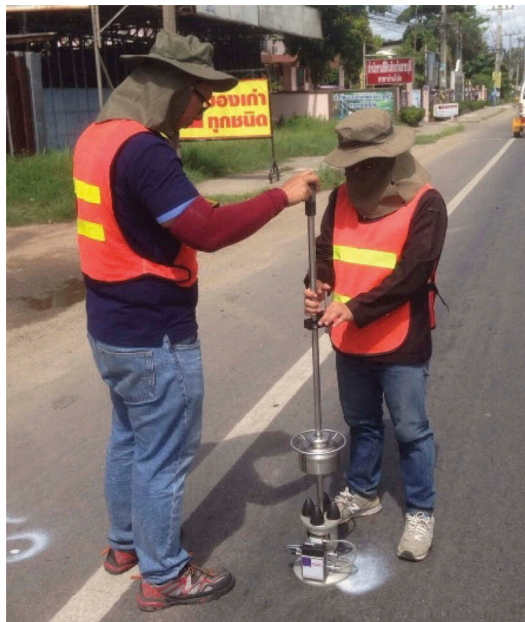
Figure 2. Light Weight Deflectometer (LWD).
