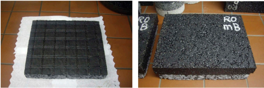
Figure 7. Pre cracked specimen with asphalt reinforcement.
