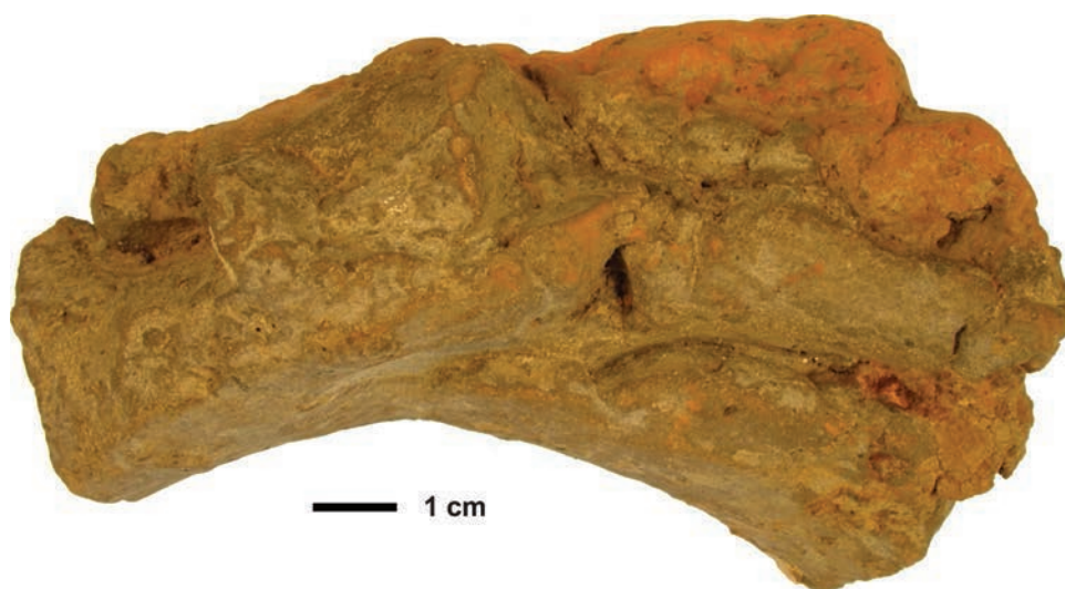
Fig 7.4 A piece of furnace structure in the form of a possible 'vent', which may have been used to allow gases to escape and the temperature to be regulated (scale c 1:1) (photo: C Steele)
