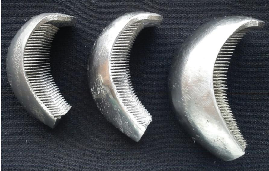
**FIGURE 3.51** A range of sizes designed (CAD) and manufactured in the SLM technology of working prototype of partial resurfacing knee arthroplasty endoprostheses with the MSC-Scaffold.
