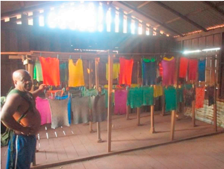
FIGURE 2 Chemist showing natural rubber sheets drying after being coloured. Photo: Tiago Muniz.
