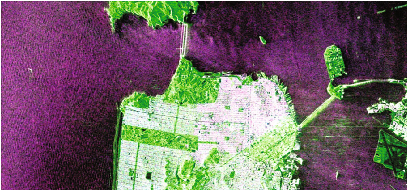
Fig. 1.8 RADARSAT-2 polarimetric RGB image over San Francisco (USA) where the colour code is S_{hh} blue, S_{vv} red and S_{hv} green. Filtered image with the LLMSE speckle filter
