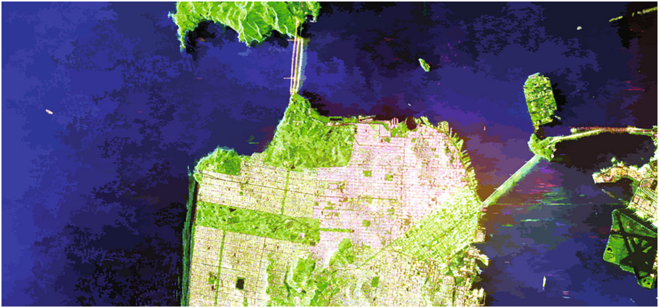
Fig. 1.9 RADARSAT-2 polarimetric RGB image over San Francisco (USA) where the colour code is S_{hh} blue, S_{vv} red and S_{hv} green. Filtered image with the BPT speckle filter
