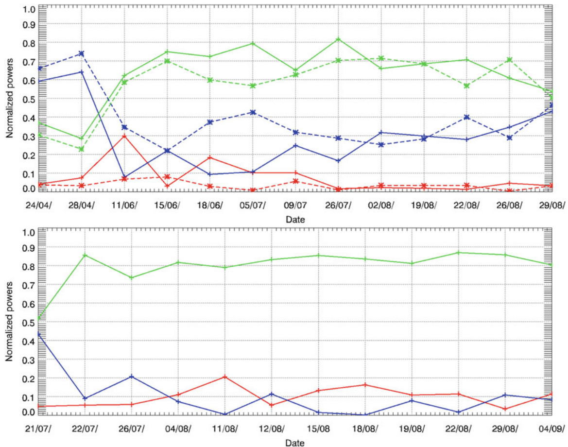
Fig. 3.8 Normalised decomposed scattering power components (red, dihedral; green, volume; blue, surface) from the model-based polarimetric decomposition for the Flevoland test sites (site 1, Plus sign; site 2, Star sign from the beginning of the observation cycle at 11th of June
