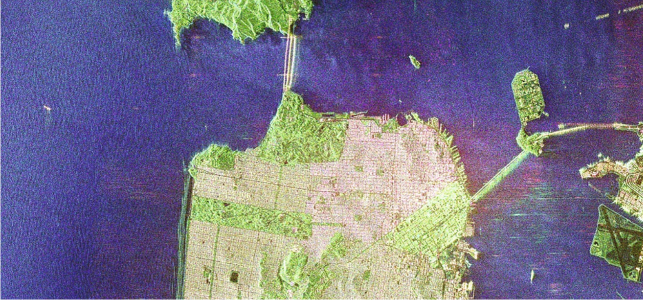
Fig. 1.10 RADARSAT-2 polarimetric RGB-Pauli image over San Francisco (USA) where the colour code is |S_{hh} + S_{vv}|^2 blue, |S_{hh} - S_{vv}|^2 red and 2|S_{hv}|^2 green
