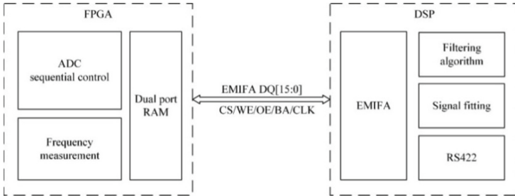
Fig. 4. Main control module.
