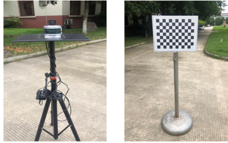
Fig. 9. Schematic diagram of placing lidar, camera and calibration plate
