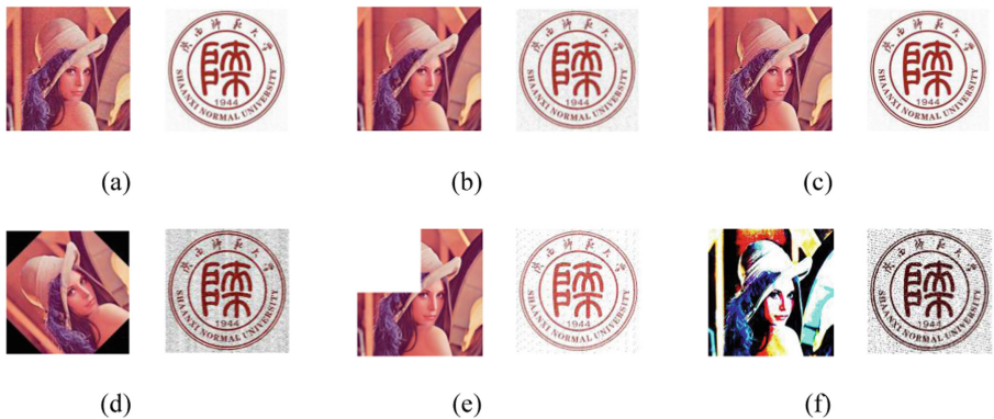
Fig. 7. The attacked watermarked image (Lena) and extracted watermark under attacks (a) Gaussian noise (b) Median filter (c) Sharpening (d) Rotation (e) Cut (f) Histogram Equalization
