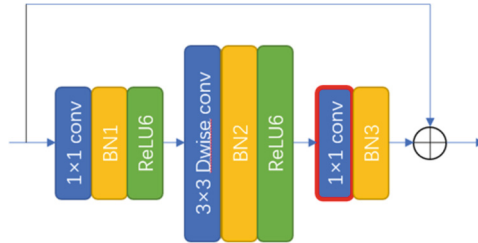
Fig. 2. The Inverted Residuals Block
