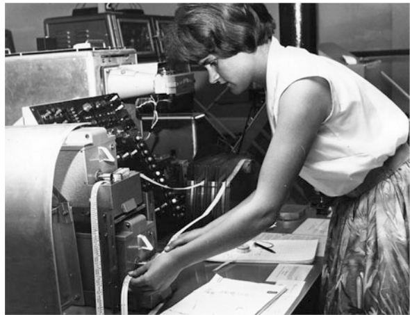
Fig. 37.14 1962 Ann Neville feeding paper tapes from Cambridge observations for the North Pole Survey into EDSAC II (CavMag, issue 11, p. 11). Courtesy of and copyright: Cavendish Laboratory, University of Cambridge. All rights reserved
