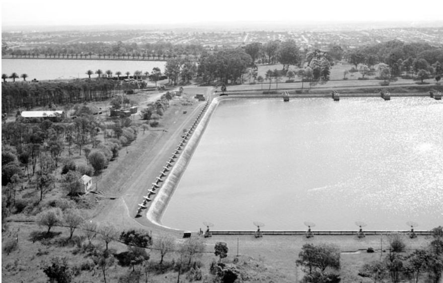
Fig. 37.10 Aerial view of the Potts Hill grating array in 1954 showing the N-S and E-W arms. NS arm is in the foreground (16 dishes) and the EW arm in the centre has 32 dishes. Credit: CSIRO Radio Astronomy Image Archive 3475-4
